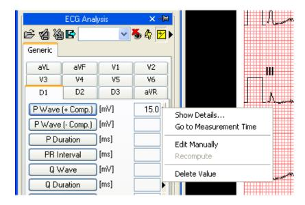
By clicking on the little arrow and then on *Show Details*, a window will be displayed in which all the samples taken for that item are shown together with the average and the standard deviation.
