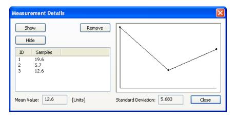
You may delete a measured value if it seems incorrect by simply selecting it and clicking the *Remove* button. Use the *Show* and *Hide* buttons to show or hide the measurements on the image.
