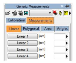
Linear, polygonal, area and angle measurements are available for rapid verification purposes.
