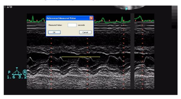
On the image, the mouse pointer will change into a pen and allow you to trace a segment. Click the left button once at the start point and then a second time at the end point. When finished, a dialogue window will prompt you to enter the dimension of the traced segment in the suitable unit of measurement.
